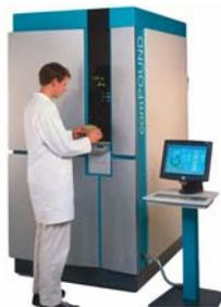
Up to 4 comPOUND modules may be linked to a comPANION remote delivery system. This allows the storage modules to be located up to 15m away from where the microtubes are delivered, in a different room – or even on a different floor.
