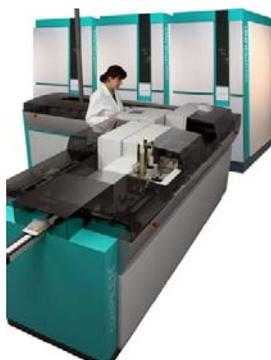
comPILER connects up to 12 comPOUND modules to provide fully automated storage and cherry-picked plate creation with no operator intervention. Together, these give rapid access to a library of up to 1.2 million samples.
