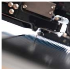
Single mosquito tip addressing a 1,536 well microplate
