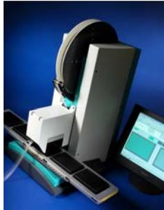
mosquito® is a low volume liquid handling instrument combining a low-cost disposable tip system with a positive displacement pipette to ensure zero cross-contamination.
