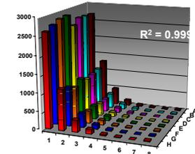
Serial dilutions in a 384-well plate. Dilution volumes - 315nL fluorescein; 685nL PBS in a ShallowWell Nunc plate.
