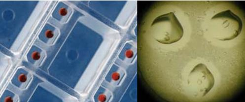
mosquito's accuracy and repeatability allows users to create several multi-component drops per well - even in high density 96-well hanging drop setups (see image above right). Such drops allow different constructs, volume ratios or protein concentrations to be assessed at the same time. This can yield 288 conditions in a single sitting or hanging drop plate.
