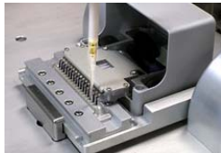
Figure 2. PatchXpress fluidics system. Photograph of the pipetting robot and 16-channel wash station.
