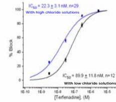
Figure 5. Effect of saline solution composition on IC<sub>50</sub> values. High-chloride internal solutions provide the best IC<sub>50</sub> values.
