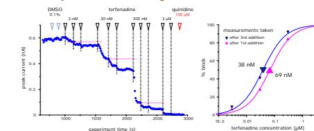
Figure 6. Use multiple additions of the same compound and concentration. The IC<sub>50</sub> value for terfenadine was 1.8-fold higher when the measurements were taken from the first addition versus the third addition. Adding compound multiple times at each concentration to mimic continuous flow conditions enables the PatchXpress 7000A system to achieve the best IC<sub>50</sub> values.
