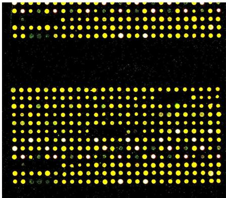
DNA microarray printed with 50  $\mu$ m silicon pins on Corning Epoxide slides using an OmniGrid 100 microarrayer
