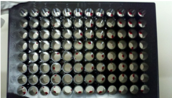
Figure 4a. Photo of residual volume remaining after sample aspiration in an MVS verification plate.
