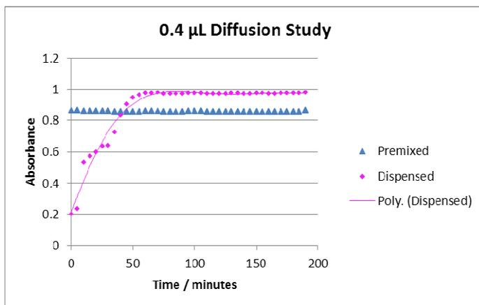
**Figure 2.** Diffusional mixing of 0.4 µL Range E solution into 200 µL of Diluent in a 96-well microplate takes more than 90 minutes before a homogeneous mixture is achieved.
