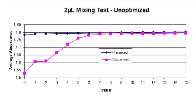
**Figure 4.** The unoptimized mixing protocol for a 384 well microplate at 2200 RPM takes around 8 minutes before consistent absorbance values are achieved.
