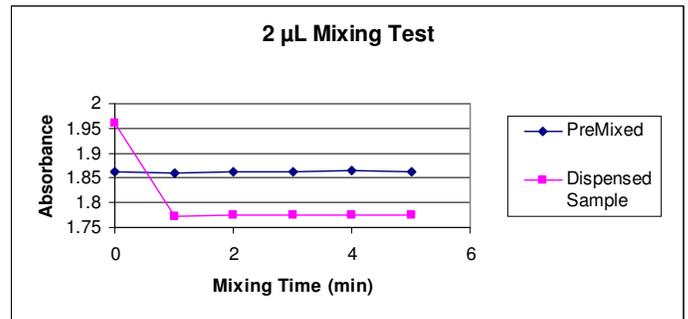
**Figure 6.** Mixing of the 2 µL sample in 53 µL of Diluent was achieved in 1 minute as illustrated by the consistent %CV values recorded after the initial, unmixed absorbance measurement. The mixing cycle duration was 60 seconds for each trial and speed was 2600 RPM. Control wells show consistent absorbance values for all measurements, as expected.
