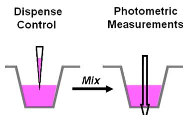
**Figure 1. 55  $\mu$ L of pre-mixed control solution was added to a portion of the microplates during testing.**
