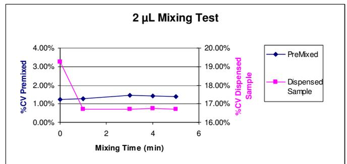
**Figure 7.** Control wells show consistent %CV values for all measurements, corresponding to the left y-axis. Test wells show consistent %CV values after 1 minute of mixing at 2600 RPM corresponding to the right y-axis.
