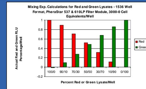
Figure 4 Graph showing comparison of actual separation of red and green luminescent signals to ideal separation percentages. Lysates dispensed using the Equator NS808 and analysed using the BMG LABTECH PHERAstar were dispensed at 100/0, 90/10, 70/30, 50/50, 30/70, 10/90 and 0/100 percentage concentrations of red and green luciferase lysate respectively. Ideal RLU percentages equal the percent of red and green lysate added per well
